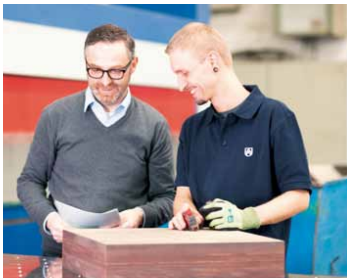
Block made from Lignostone®: only selected red beech veneers of the highest quality are used for production
