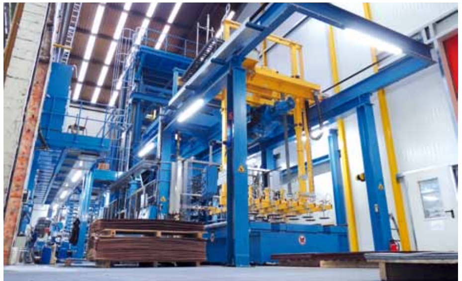
State-of-the-art: new press for the production of Lignostone® sheets
